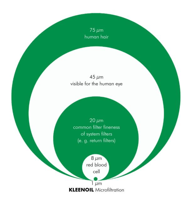
Most of the contamination in oil that can damage a machine is not visible to the naked eye. The necessity to filter the oil down to 1 micron filter fineness results from the fact, that narrowest fits e.g. in hydraulic pumps, control valves and seal clearances in parts, are only one or a few micron.
