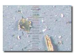
Imminent total breakdown, high wear, malfunctions at pumps and valves, damage of seals
