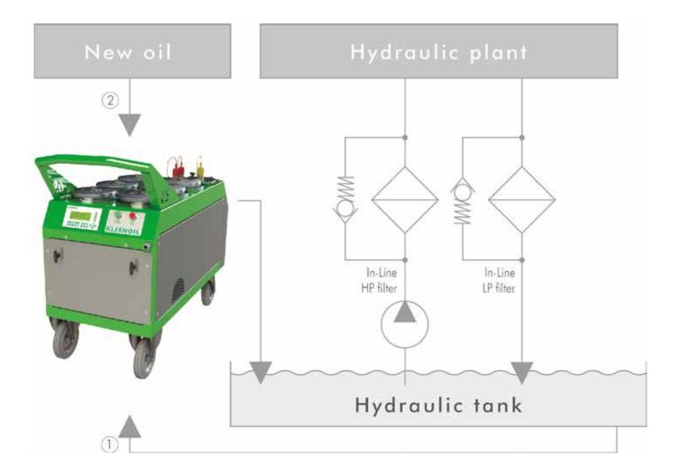
Duration and frequency of the filtration are dependent on the level of fluid contamination, the type of construction and the employment of the machine. It is important to observe that during the filtration all system functions have to be carried out intensely and frequently enough. Only if during the filtration time the entire system volume is circulated several times it can be ensured, that the contamination in the oil is removed by the filtration system.
