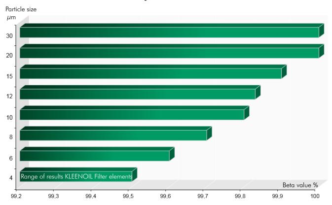
The efficiency of a filter element is not only determined by the filter fineness, but also by the retention capacity. The result is indicated as beta ( $\beta$ ) value. The beta value and the filtration fineness are indicated in relation to each other in the result. Due to lack of measuring possibilities with calibrated particles  $< 4 \,\mu\text{m}$  in this case  $4 \,\mu\text{m}$  particles are also used and the filtration fineness  $< 4 \,\mu\text{m}$  is determined arithmetically.
